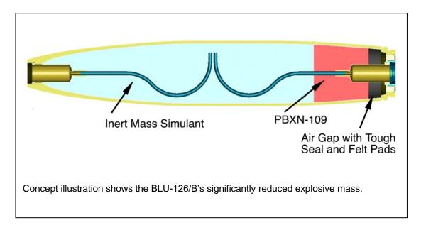
The proposed BLU-126/B design solution was developed under the following constraints:
